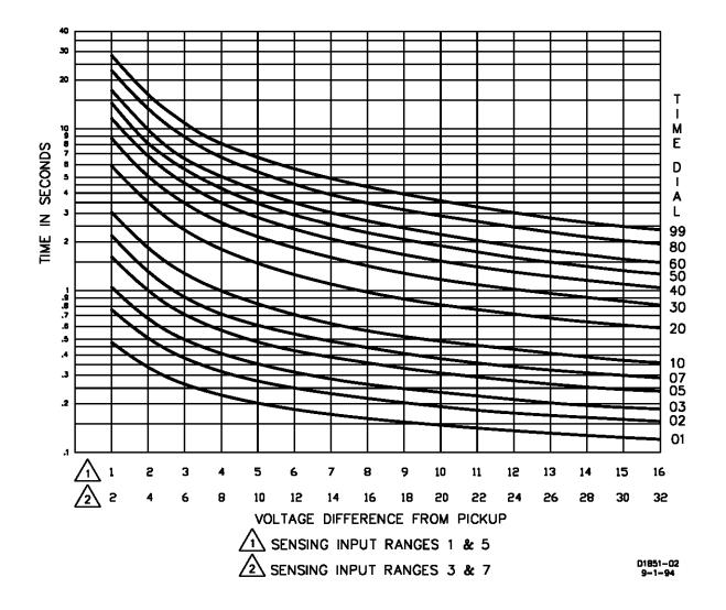
Figure 1-3. Overvoltage Inverse Time Curves, Low Ranges (Drawing Number 99-1510)
