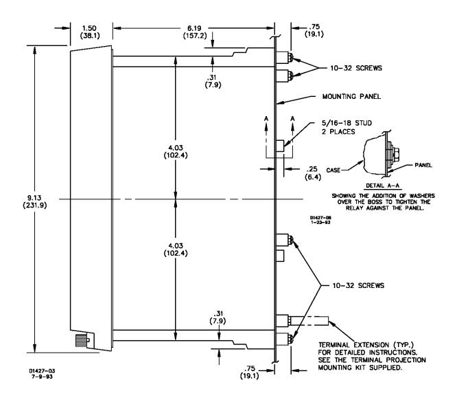
Figure 4-7. S1 Case, Double-Ended, Projection Mounting, Side View
