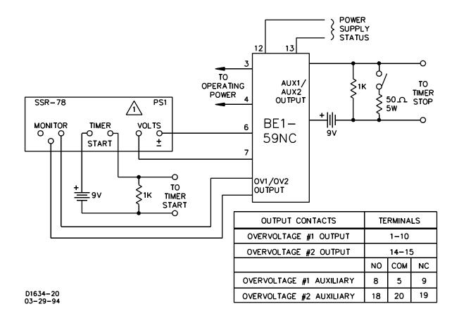
Figure 5-1. Typical Test Setup Timing Option E2
