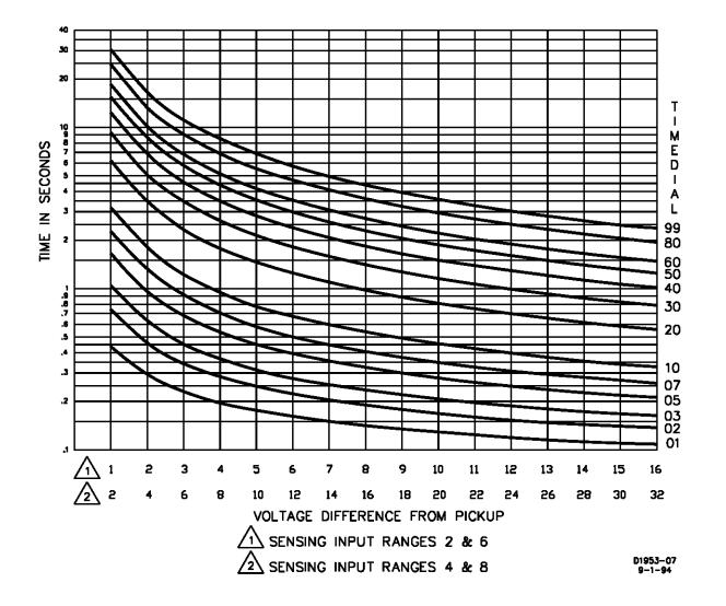
Figure 1-4. Overvoltage Inverse Time Curves, High Ranges (Drawing Number 99-1545)
