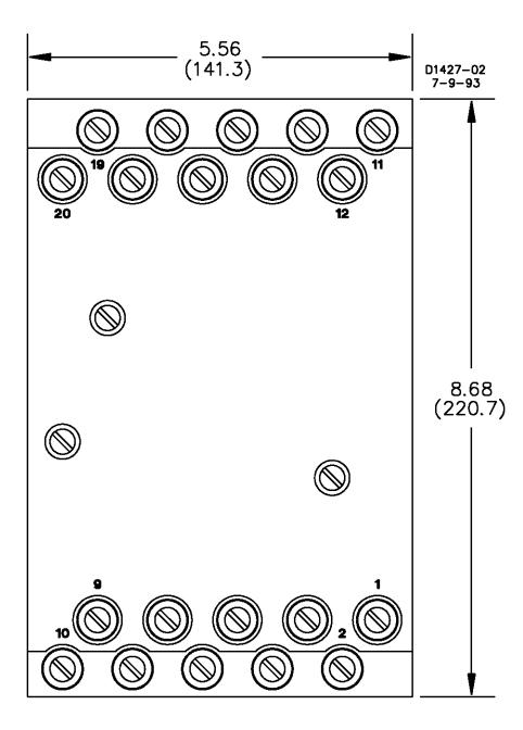
Figure 4-6. S1 Case, Double-Ended, Projection Mounting, Rear View
