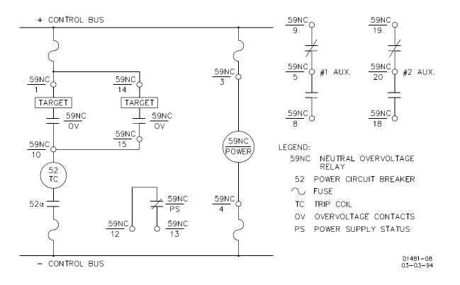
Figure 4-8. Typical Control Circuit Connections
