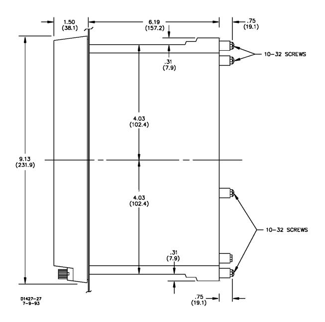
Figure 4-3. S1 Case, Double-Ended, Semi-Flush Mounting, Side View
