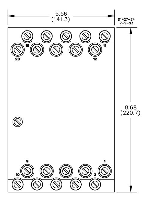
Figure 4-4. S1 Case, Double-Ended, Semi-Flush Mounting, Outline Dimensions, Rear View
