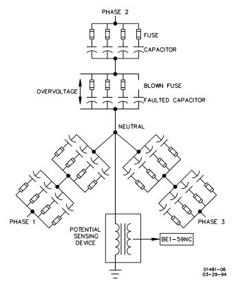
Figure 1-1. Ungrounded 3-Phase, 3-Wire System
