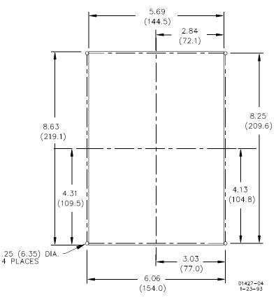
Figure 4-1. S1 Case, Panel Drilling Diagram, Semi-Flush Mounting
